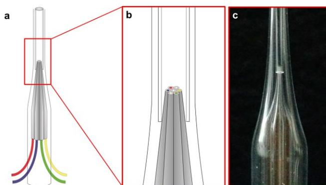
Figure 1. (a) Schematic of the pulled multibarrel capillary device with oil and water input tubing, (b) magnified view of the pulled end of the capillary bundle, and (c) image of an assembled device.
