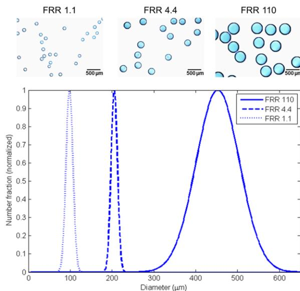
*Figure 3. Size distributions for droplets formed using a single capillary within the multibarrel system as a function of flow rate ratio (FRR), defined as the ratio of dispersed:continuous flow rates.*
