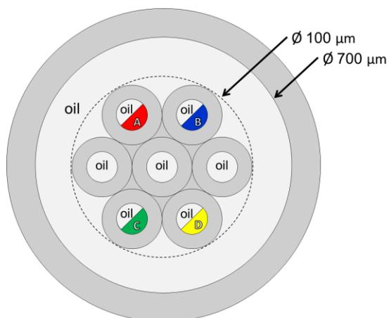
*Figure 2. Configuration of inlets: the 7-barrel capillary contains 3 center inlets which are connected to oil phase and two sets of adjacent capillaries connected to oil and water (A,B,C,D) phases separated by a valve, enabling rapid switching between phases for digital control over droplet formation for programmable emulsions.*
