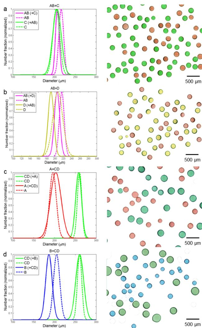
Figure 4. Size distributions of single and dual droplets formed simultaneously, compared to each droplet type when formed alone.
