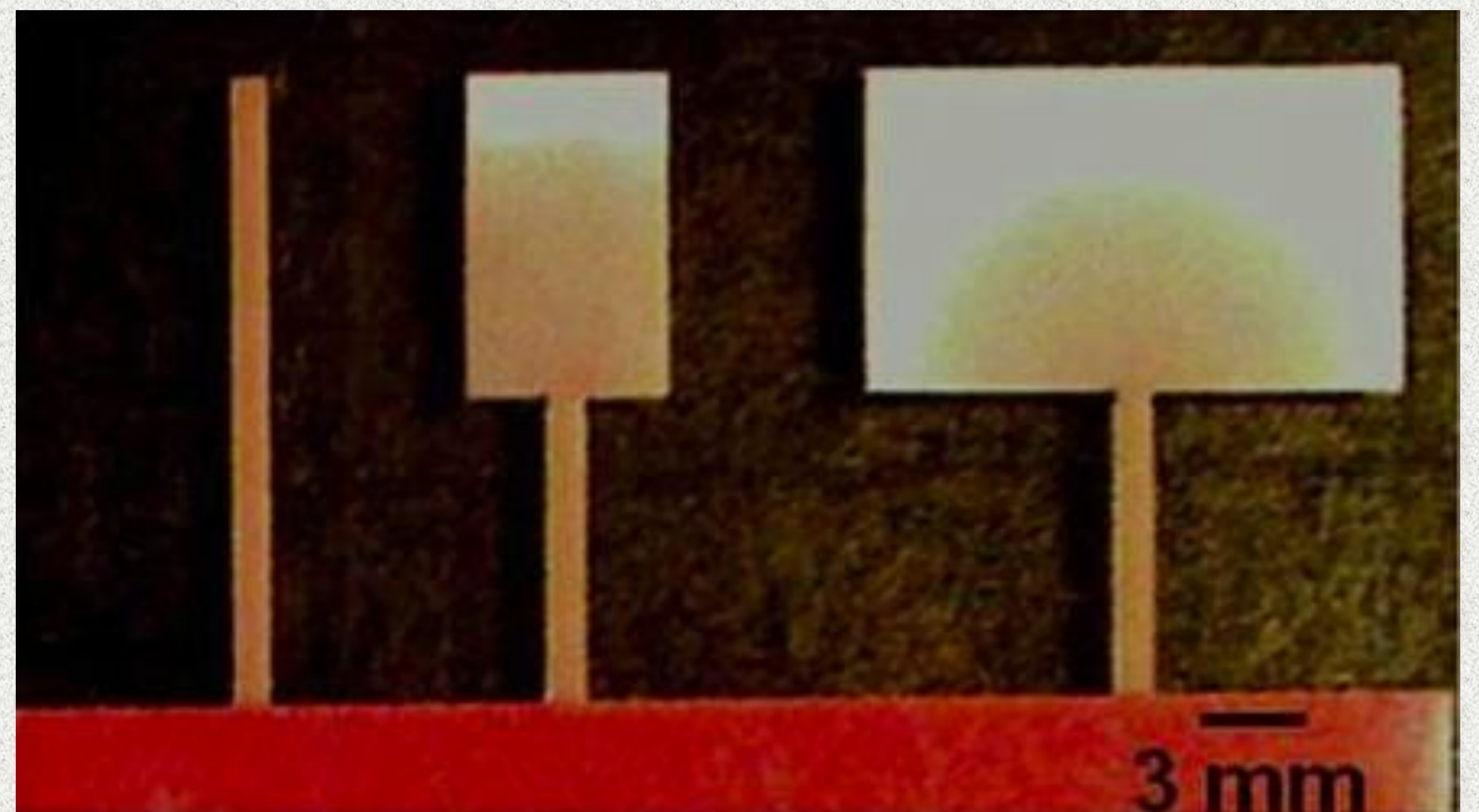
Flow of liquid in paper microfluidics networks with different width expansions. Picture from: Microfluidics 2.0 workshop , http://www.mf20.org/microfluidics-20-toolkit/controlling-flow-rates-paper-networks
